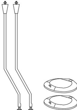
Two floor-stand posts, with "knurled" nuts, cone-shaped fittings, and 19mm-long hex head bolts installed.
