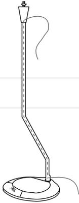
“Fish” the speaker wire through the stand posts and bring it out through the round hole on the cone-shaped fitting.
