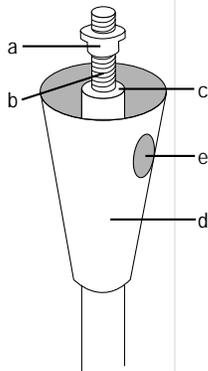
Be careful when starting the threads to avoid cross-threading (misaligning the threads – see Step 3); cross-threading may damage the speaker and/or the stand.
